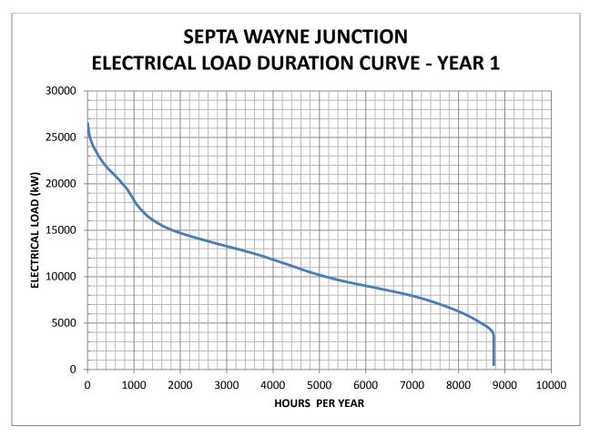
The electrical load duration curve below is based on the projected year one electrical load at Wayne Junction.
